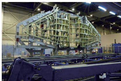
图2 机翼/机身整体大部件 Fig.2 Large integral structure of blended-wing-body
